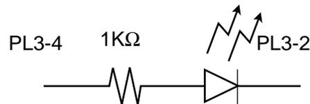
Fig. 1—Blinky Light Schematic
