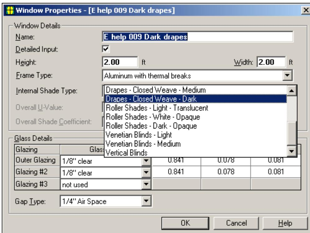
**Figure 1 – Window Properties Detailed Input Screen Showing Internal Shade Choices**
