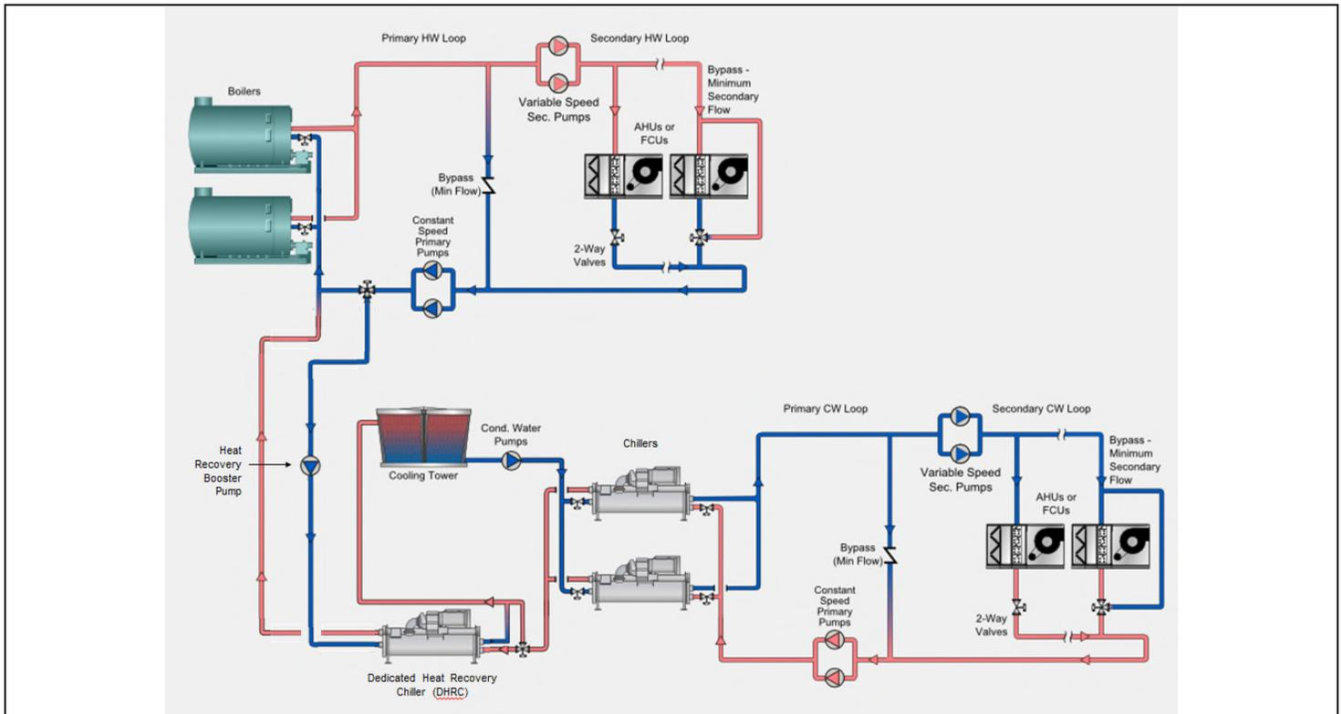
Figure 1. Diagram of Heat Recovery Plant with DHRC in Condenser Loop
