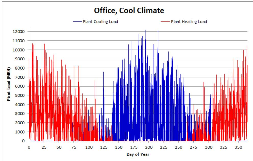
Figure 3. Building with Poor Heat Recovery Potential
