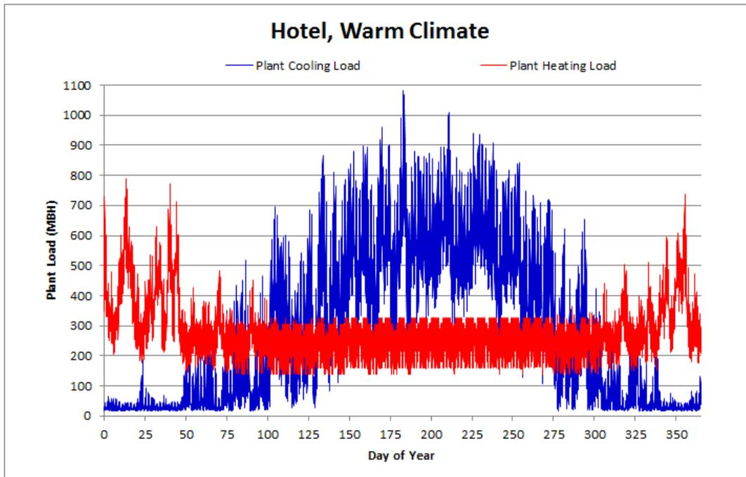
Figure 2. Building with Good Heat Recovery Potential
