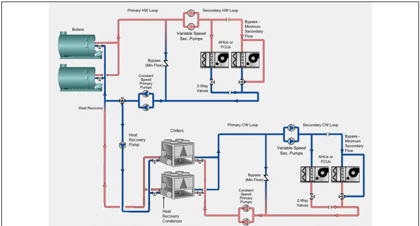
Figure 1. Diagram of Heat Recovery Plant with Air-Cooled Chillers with Heat Recovery Condensers
