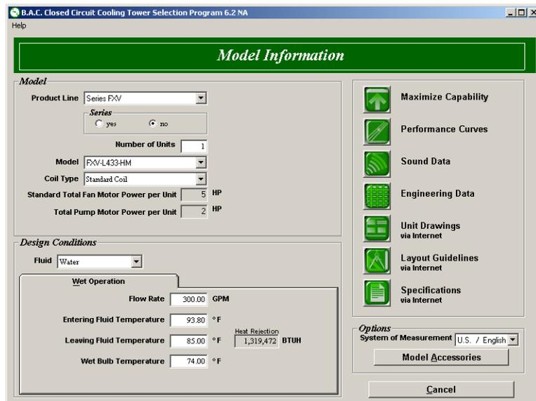
Figure 17 – Cooling Tower Selection
