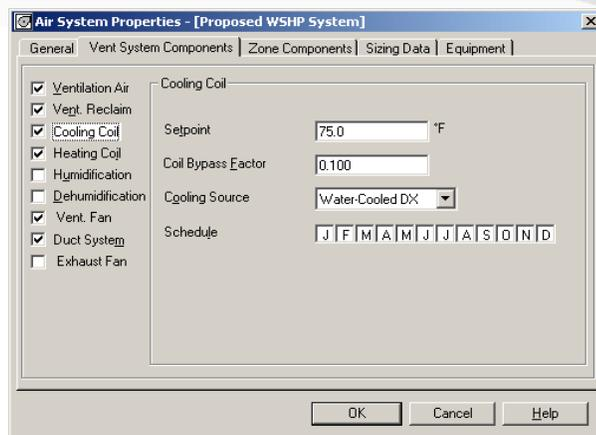
Figure 4 – Common Ventilation System Properties
