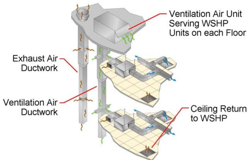
Figure 2 – Common Ventilation System for WSHP
