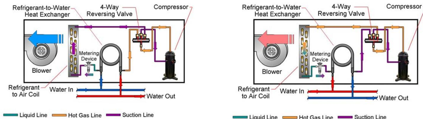
**Figure 1 – WSHP Cooling & Heating Operation**
