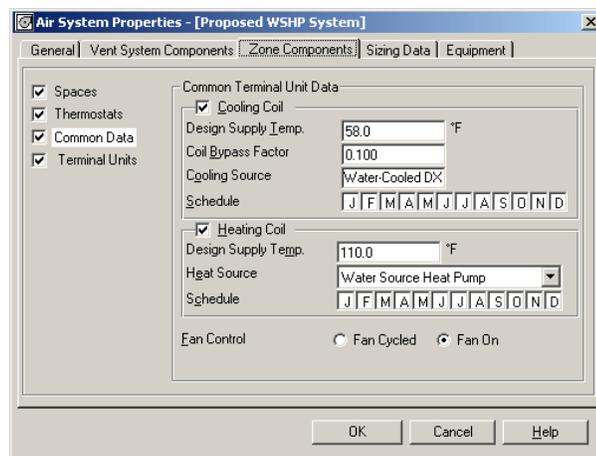
Figure 5 – Common Data for WSHP
