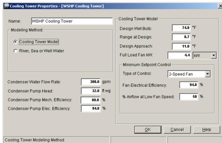
Figure 18 – Cooling Tower Properties Input
