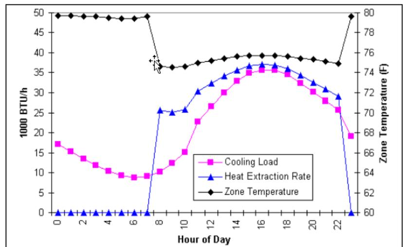
Figure 6 - Load, Heat Extraction, and Room Temperature Profiles
