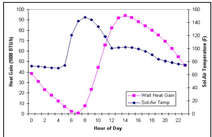
Figure 2 - Wall Heat Gain Example
