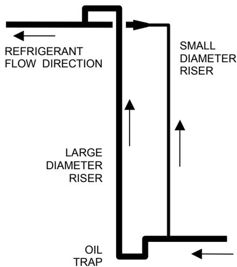
Figure 2. Typical Double Riser Arrangement
