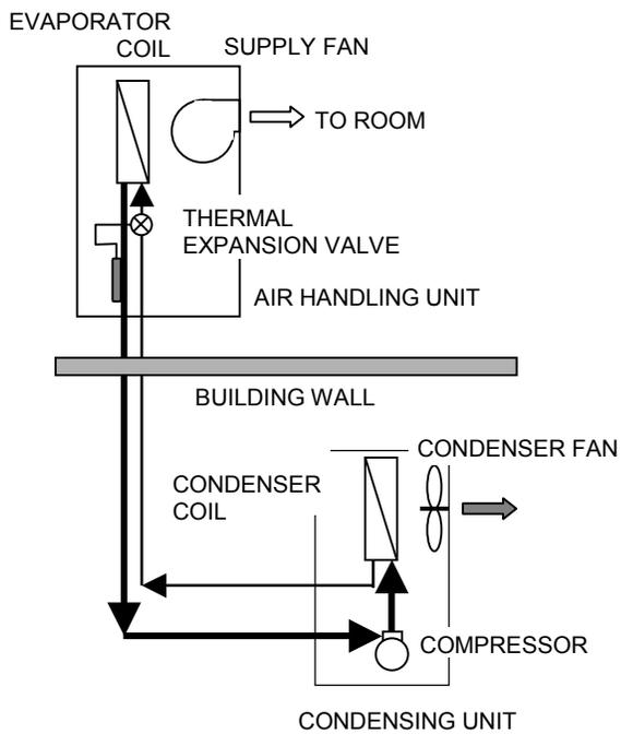
Figure 1. Typical Split System Schematic
